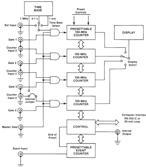
Fig. 1. ORTEC Model 974A Counter/Timer Architecture.
